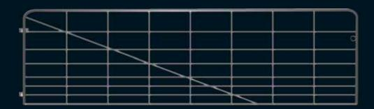
Height 1.05 m Frame 25 NB Fixed Lug 20 mm Adj. Lug 20 mm Horizontal 6 bars 7.5 mm Diagonal 6.3 mm 1 bar (1.83 m - 4.27 m) 2 bars (4.57 m, 4.87 m) Vertical 25 x 3 mm 3 bars (1.83 m) 4 bars (2.13 m, 2.44 m) 5 bars (2.74 m, 3.05 m) 6 bars (3.35 m) 7 bars (3.66 m) 8 bars (3.96 m, 4.27 m) 9 bars (4.57 m, 4.87 m)
