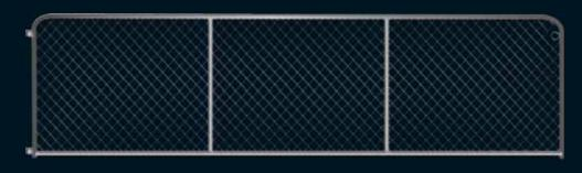
Height 1 m Frame 25 NB Fixed Lug 20 mm x 2 Chainlink 75 x 3.15 mm Vertical 25 NB 1 bar (1.83 m, 2.13 m) 2 bars (2.44 m - 4.87 m)
